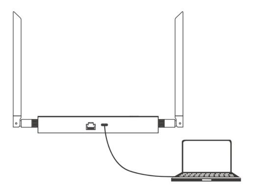
Use a Type-C charging cable: connect one end to the device's Type-C port, and the other end to the host device.
