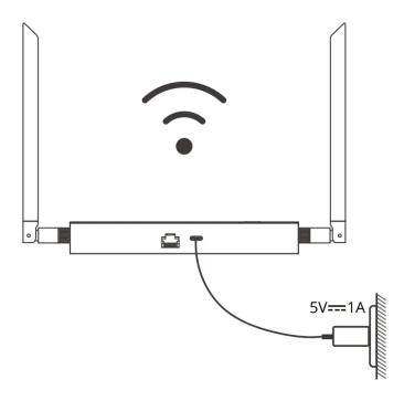
Use a Type-C charging cable: connect one end to the device's Type-C port, and the other end to a power adapter. Plug an RJ45 Ethernet cable into the network port and connect it to the router.
