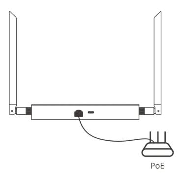
1. Connect the device to a PoE-enabled router, switch, or PoE power module using an RJ45 Ethernet cable. This completes the power connection.
